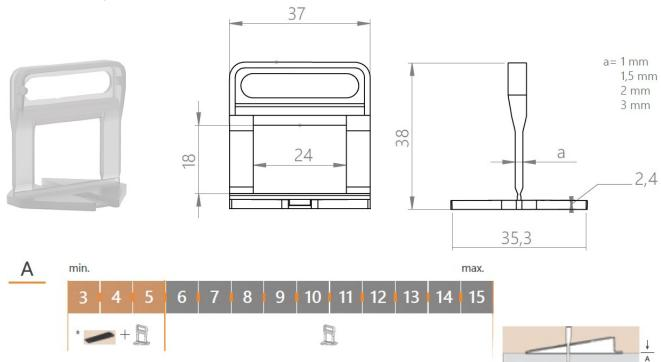
Spacer clips are used for all tiles with a thickness from 3 mm up to 15 mm. (\*) Wedge Separator must be used with tiles thinner than 6 mm.
